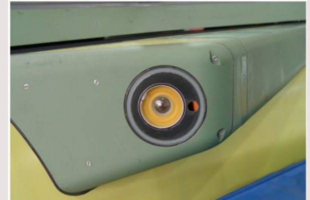
Existing CMWS(V)1 EOMS Installation
